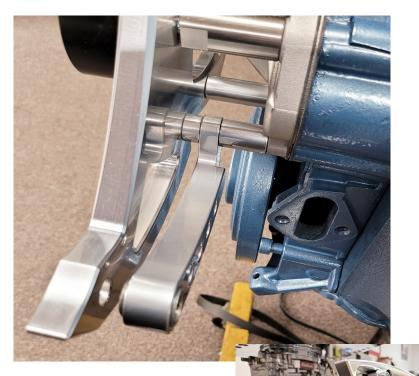
Install (13148A-09) rear support bracket to water pump as shown in photo using a (TP3-1.100") spacer in between rear bracket and pump and in between rear bracket and main bracket use a (TP3-.400") spacer. Retain with a (S166) 5/16-18 x 3.5" shcs. Leave loose. Next install (S453) 5/8-18 x .850" set screw. Make sure hex is facing engine.
