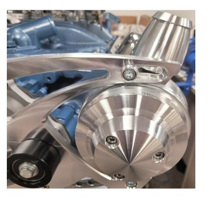
Now install the alternator fan (221-A) and pulley (206-A) to the alternator. Use (S685) 11/16 " lock washer and install alternator nut. We recommend an impact driver to install. Now install the alternator pulley cover (306-A) to the pulley using three (S028) 8-32 x 1" shcs.
