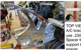
TOP VIEW A/C bracket use .2300 Spacer then rear support then.312 spacer
