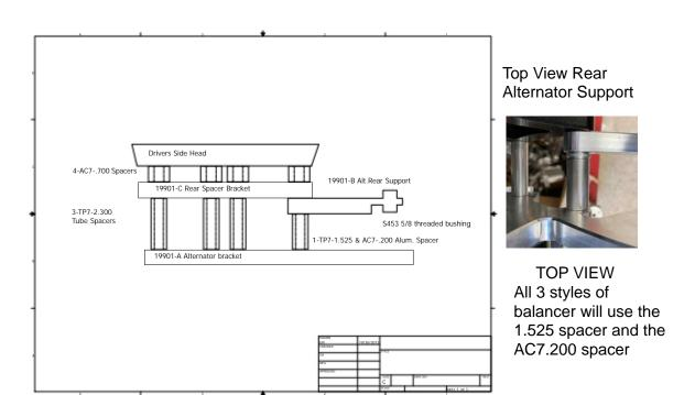
Install the alternator (P581) to the alternator bracket. In the upper hole use a M8 x 25mm SHCS (S551). In the lower mounting hole use a 5/16 x 3-1/2" " shcs (S166). Install bolt thru the front bracket then thru the alternator making sure the rear adjuster screw is threaded forward to where it is contacting on the back of the alternator ear. Secure with a (S660) 5/16 washer and a (616) 5/16 lock nut.
