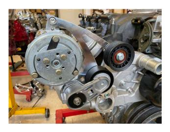
Install the a/c compressor (P425) to the rear side of the a/c bracket using two (S551) M8 x 25mm shcs. Attach the rear a/c support bracket (19902-B) to the a/c lower ear using a (S213) 5/16 x 1-1/2 " hex bolt and two (S660) 5/16 washers and a (S616) 5/16 lock nut. Now add a Ribbed idler (P761) to the upper tapped hole of the a/c bracket using a (S322) 3/8 x 1-1/2" hex bolt and a (S666) 3/8 washer.
