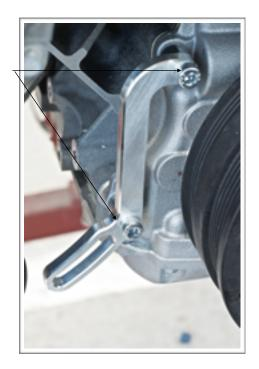
Mount the belt tensioner (P753) to the water pump tangs on the passenger side using (2) M10 x 30 MM SHCS (S561).
