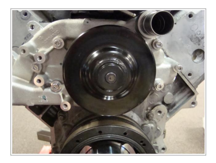
Mount the alternator (P587) in the upper outer hole just below the drivers head. Use a M10 x 80 MM SHCS (S562) and space the alternator from the block using a (AC7-.312) aluminum spacer as shown.
