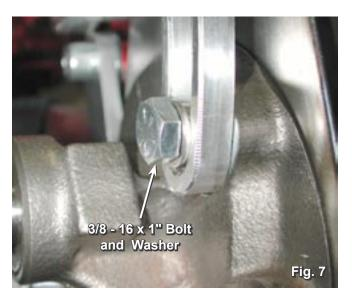
8. Mount power steering pulley to power steering pump shaft. Check power steering pulley to crank pulley alignment. Install belt (*Use 39.5" 5 rib serpentine belt for serpentine conversions*) and adjust belt tension by pulling up on the power steering pump. Belt tension is correct when there is no more than ¼" play in the belt at midpoint between the power steering pulley & the crank pulley. Lock the belt tension by tightening the adjustment bolt with a 9/16" opened end wrench (fig. 8).
