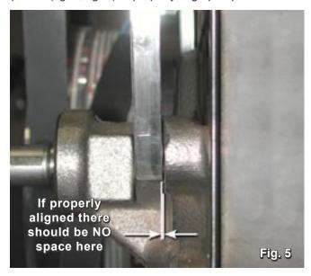
Important Note: Due to variations of water pump boss castings particularly in aftermarket and polished pumps it may be necessary to add spacer washers between (20176-A) Front Support Bracket and the water pump boss. (fig. 6) ['Apacer washer between the (20176-B) Rear Sup] ['c O'a&\^o\angle a'f\_[, ^\A\c^\\angle a'A\c^\\angle a'f\_] \tilde A\cappa a'f\_] \ A\co\angle a'f\_A\co\angle a'f\_A\co\angle
