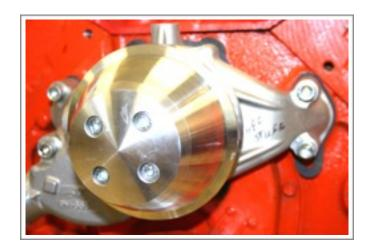
**Photo-6**Install the Water pump pulley (6222-A)
