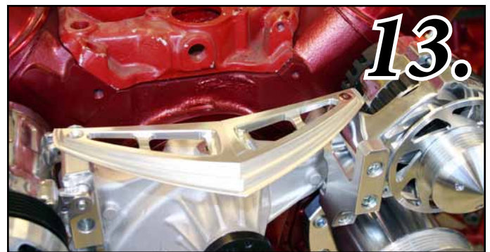
Photo-14 . Mount Water Pump Pulley (7667) & Water Pump Nose Cover (332) to Water Pump using four (4) \frac{5}{16} "-24 x 1\frac{1}{2} " socket head cap screws. Also install the A/C cover .
