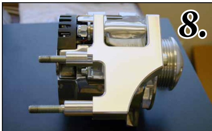
Photo-9 Installing the Alternator Bracket, use a \frac{3}{8} x 3\frac{3}{4} " SHCS (Lower Hole) and a \frac{3}{8} x 5\frac{1}{2} " (upper hole) thru the water pump. And into the block as Shown.
