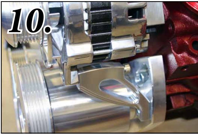
Photo -11 Installing the A/C unit to the A/C mounting bracket, Use a 8mm x 100 mm Hex bolt thru the rear of the A/C unit Noting the A/C unit mounts to the left side of the bracket.
