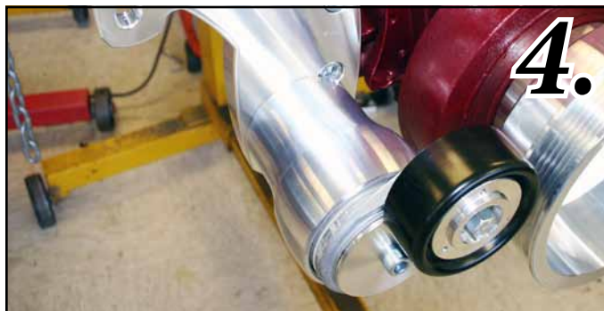
Photo-5 Mount the power steering Spacer Bracket (20357-C) & Power Steering Housing Cover (20357-B) and the power Steering pump together using (2) M8 x 1.25 x \frac{3}{4} " SHCS.
