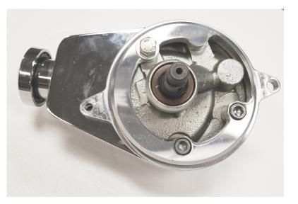
Step-5 Install (21074-A) power steering adapter bracket to (P304) power steering pump with two (S244) 3/8-16 x .75" shcs and one (S311) 3/8-16 x .75" hex head and a (S667) 3/8 x 5/8" washer under the head of bolt as shown.
