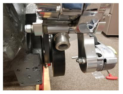
Install (P555) alternator with a (S280) 3/8-16 x 5.5" shcs and a (TP3-1.775") long spacer in between alternator ear and (S450) set screw. Adjust (S450) to take up any gap. Secure with a (S622) 3/8-16 lock nut.
