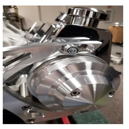
In the upper slot of main bracket install a (MM100) bolt bushing and a (S146) 5/16-18 x 1" shcs. Now install (629-A) power steering pulley on to pump. Make sure woodruff key does not slide up on shaft and that pulley is perfectly seated back. Failure to do so can cause premature failure of pulley. Secure with power steering nut provided with pump. Now install power steering pulley nose cover (360-A) with three (S106) 1/4-20 x 1.25" shcs.
