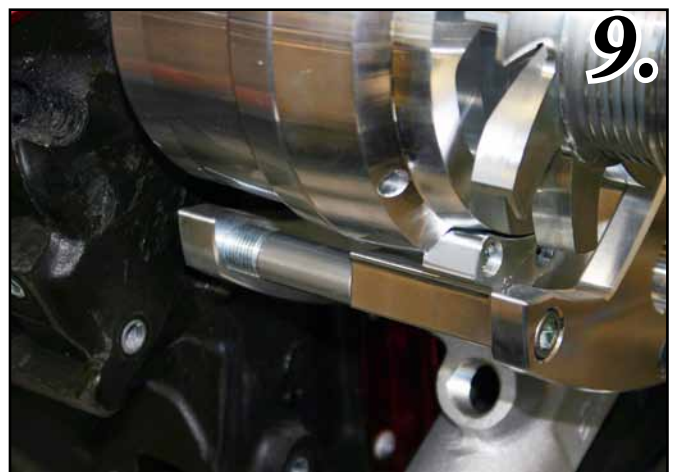
Fig. 10. In the upper Alternator and Power Steering slots use the two (MM100) Alum. Bolt bushings and the (2) \frac{5}{16} x 1" (S146)
