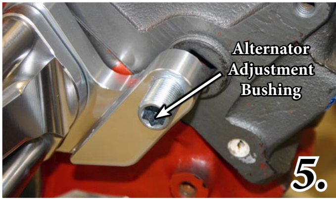
Photo-6 Using one \frac{3}{8} \times 4\frac{3}{4} " SHCS (S277) through the Main Bracket, install the Alternator (P572), Put a .700 spacer (TP3-.700) behind the alternator mounting ear and adjust the Adjustment Spacer (S450) so its tight to the back of the alternator. In the upper slot use a MM100 Bushing and a M8 x 1.25 x 35mm SHCS (S553).
