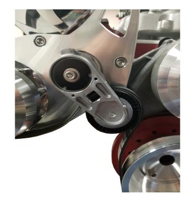
**Step 13**To install belt, use a 1/2" drive ratchet and rotate clockwise and install a 82.5" 6 rib belt and route belt as shown below. We recommend **Dayco part # 5060825**.
