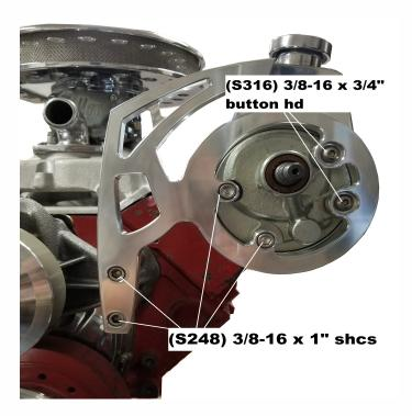
Install (25114B-08) to outer cylinder head bolt with a (S322) 3/8-16 x 1 1/2" hex bolt and a (S666) 3/8 x 3/4" washer. In between bracket and cylinder head use a (TP3-.300) spacer. Now tighten the front main power steering bracket bolts and then the two rear support bracket bolts. **Note: due to variations in cylinder heads it may be necessary to add shims to rear support bracket.**
