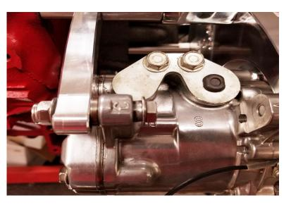
**Step 8** Install (221A-08) alternator fan, (206A-08) alternator pulley and provided (S685) lock washer with alternator nut. Use impact to secure nut or torque to 90 lbs.
