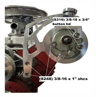
Install (25114-B) to outer cylinder head bolt with a (S322) 3/8-16 x 1 1/2" hex bolt and a (S666) 3/8 x 3/4" washer. In between bracket and cylinder head use a (TP3-.300) spacer. Now tighten the front main power steering bracket bolts and then the two rear support bracket bolts. **Note: due to variations in cylinder heads it may be necessary to add shims to rear support bracket.**
