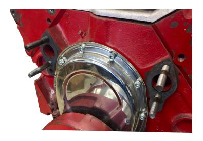
Slide the water pump (1988 to 1995 reverse rotation long water pump) over the four studs. On the passenger side install two of (S777) 3/4" o.d. x 2.820" long stainless spacers. On the driver side install two (S775) 3/4" o.d. x 2.720" stainless spacers.
