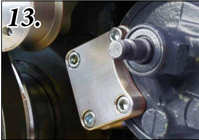
Photo -13 Install the Pump Bracket Unit to the block using the two lower drivers side holes next to the crank,
