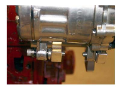
**Photo-7** Install the 5/8" Dia. Threaded bushing (S453) into the Alternator Rear Support as shown.
