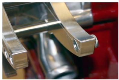
**Photo-8** Installing the Alternator (P572) using a  $\frac{3}{8}$  x  $3\frac{1}{2}$ " SHCS (S270) thru the bottom bolt hole. Adjust the  $\frac{5}{8}$ " Dia. Threaded bushing (S453) to take up any slack between the Alternator's lower mount and the Rear Alternator Support Bracket. Secure with a  $\frac{3}{8}$ " Lock nut (S622). In the upper Alternator location use a M8 x 35mm SHCS (S553) and Countersunk Aluminum Bushing (MM100). (do not tighten at this time).
