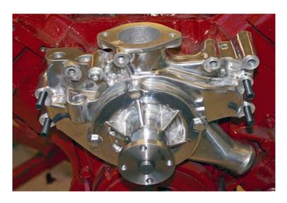
**Photo-3** Slide the A/C Rear Supports (40722-A) over the studs on the passenger and side and Alternator Rear Support (40723-A) over the stud on the drivers side. Secure using the (4)  $\frac{3}{8}$  x 2" (S771) Threaded Stainless Spacers mounting over the studs as shown.
