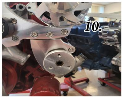
**Photo-10** On kits with Power Steering install the Power Steering Pump Unit (P313) to the Power Steering Bracket (40724-A) using (2) M8 x 25mm SHCS (S551).
