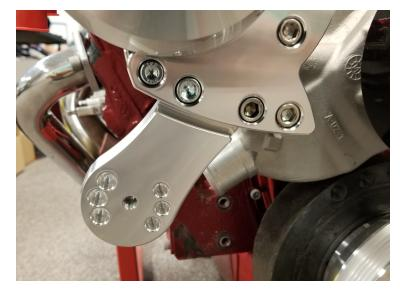
**Photo-12** Install (21124-A) tensioner bracket to main bracket on passenger side with two (S248)  $3/8-16 \times 1$ " SHCS.
