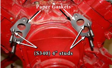
**Photo-2** Using silicon sealer and new gaskets, install the Provided Water pump (P182) over the four studs as shown.
