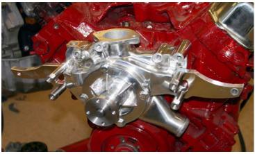
**Photo-4** Install The Main Face Plate (40741-A) using (4) (S244)  $^{3}$ /s x  $^{3}$ /4 " SHCS thru the four counter sunk bolt holes in the front of the plate and into the four Stainless Threaded Spacers.
