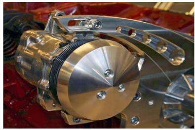
**Photo-6** Install the rear  $\frac{5}{6}$  x 2" SHCS (S155) A/C support bolt thru the rear lower ear of the A/C unit. Between the rear A/C ear and the Rear A/C support install a .200 Aluminum Bushing (AC3-.200) as shown and tighten at this time.
